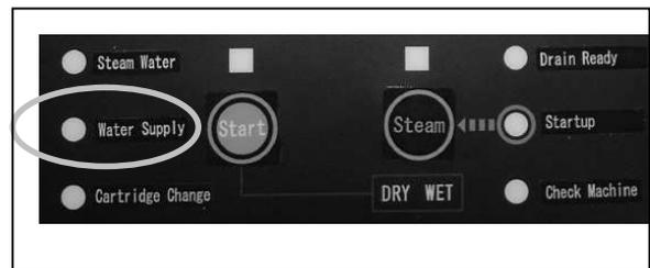
Water supply LED turns on to flashing after filling water.
