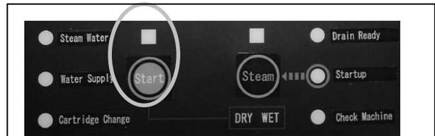
Let the machine drive for 1 hour. After 1 hour, turn OFF with pushing start switch.
