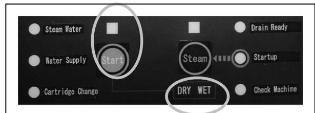
② Point the nozzle to safe place (For example a towel is good idea), press and hold the steam switch on the steam gun for 3 seconds. The gun spouts steam from the nozzle. To turn off, press the steam switch once (for short time). You can also operate this with steam switch on the control panel.
