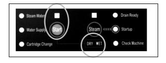
Let the machine drive for 1 hour. After 1 hour, turn OFF with pushing start switch.
