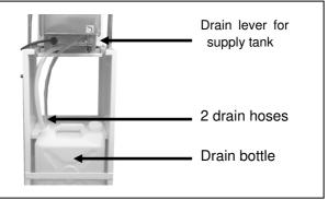
③ Close drain lever of supply tank after draining all water.
