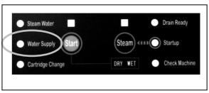
Water supply LED turns on to flashing after filling water.
