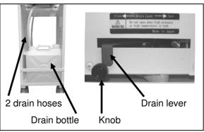
\*Do not push start switch while the drain lever is loosened. This turns on alarm and does not start.
