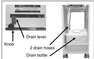
Do not open the drain lever while drain ready LED is OFF. There is still pressured steam inside of evaporator. Pressured steam will sprout from drain hose. You might burn yourself.
