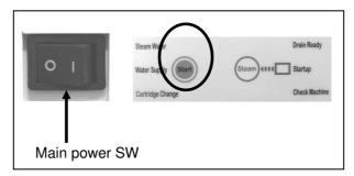
⑦ Push and hold start switch for 7 seconds. The alarm informs you that the soft water cartridge change time reset is done.
